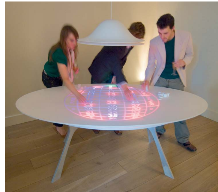
In his exhibition “The Electric Kid Show”, Moritz Waldemeyer from Germany displays tables made of Corian® with interactive game interfaces – the material is translucent and reacts to touch.
